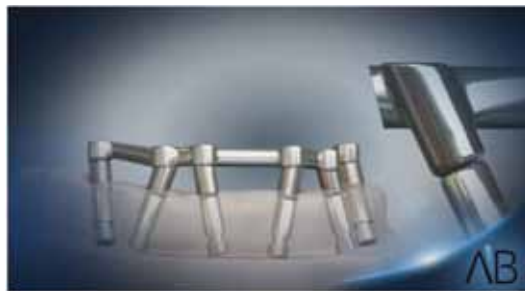
The casting is cemented to the titanium base.
